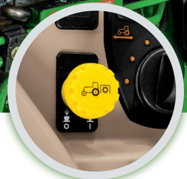
A modulated, wet disk clutch engages the PTO on both 4M and 4R models. Simply pull up on the yellow knob and the PTO gently engages
