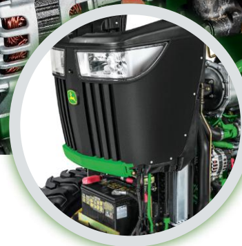
Sliding front grill allows easy service to the battery and radiator
