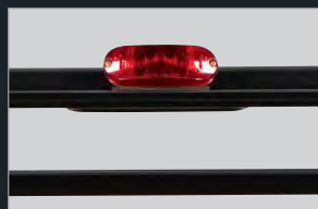
Brake/Taillight Attaches to rear bar of OPS.
