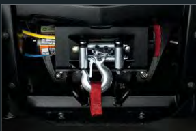
Warn® Winch 3,500 lb. (1361 kg) winch. Includes a water-resistant remote control.
