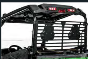
OPS Roof & Rear screen Provides additional protection from the elements and rear. Includes headrests.
