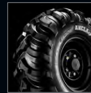
Ancla XTs for good mudding/extreme terrain Front 26x9xR12 Rear 26x11-R12
