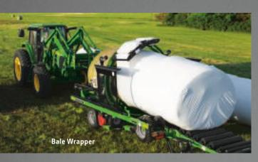
Wrap 120 bales per hour with the fast-action Frontier bale wrapper. It keeps your bales safe from harsh weather and helps seal in the nutrients for higher quality feed.
