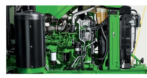
**Final Tier 4 engine** is rated at 173 hp (129 kW) and boosts power 5 percent more than our former model. This 4.5L engine is designed to increase power bulge from 173 to 182 hp (136 KW) with a 10% gain in peak torque. That's dependable power in harsh conditions to let you spray at higher speeds than before.
