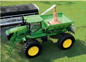
Keep spreading in the field longer. Load up to 10 tons (9,072 kg) of product in the DN485 hopper, available on the R4045 Sprayer. With the DN456 hopper, load up to 6.6 tons (6,000 kg) of product.
