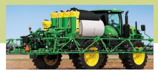
**Direct Injection system** increases your flexibility by changing rates and products on the fly without stopping to mix. Increase flexibility by changing rates and products on the fly without stopping to mix products. The integrated system injects products directly into the system at the boom. The results: quicker changeovers, increased flexibility and lowered risk of using multiple products.
