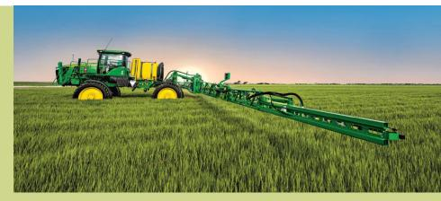
**Proven design.** We realize carbon fiber isn't ideal for all situations, and that's why we rely on the proven design of our steel booms to get the job done. The rock solid construction includes a reliable dual swing link suspension and greater stability while delivering consistent height above crop, acre after acre. And the flat-fold design lets you spray up to 120 ft. (36 m) wide, covering more acres with fewer passes.
