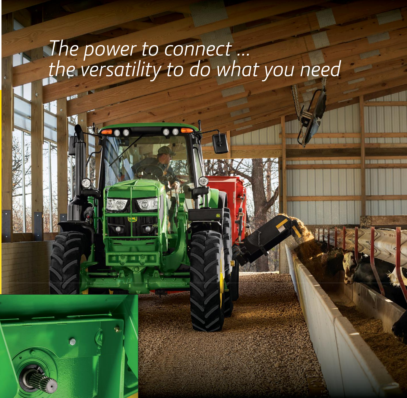
The 540/1000 RPM reversible PTO on the 6M can be removed and replaced in less than 30 seconds without a mess.
