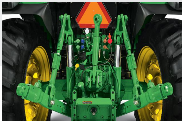
Big lift: With 30 gpm (113 lpm) and up to 10,582 pounds (4,535 kg) of hitch-lift capacity, you'll be ready for loader chores and big implements.
