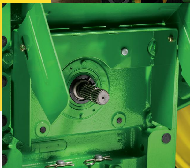
The 540/1000 RPM reversible PTO on the 6M can be removed and replaced in less than 30 seconds without a mess.
