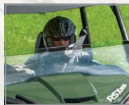
Windshields. Half (shown), full and full glass with wiper. Tool-less installation.
