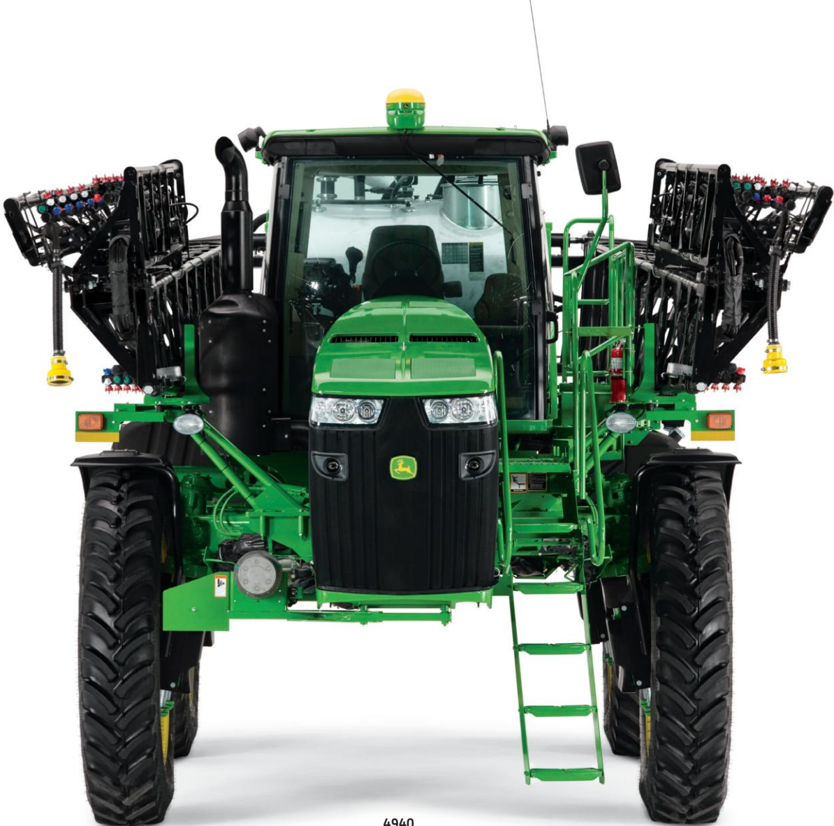
4940 1,200-gallon tank 120-foot boom Available drybox
