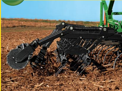
Round-bar rolling baskets on 2-bar coil-tine or flat-bar rolling baskets on 3-bar spike-tooth harrows (on selected floating hitch models and all Level-lift models) break down clods while firming soil to preserve moisture. (Round-bar rolling baskets on 2-bar coil-tine harrow shown.)
