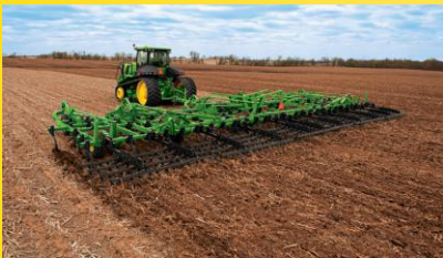
The 4-bar coil-tine harrows provides 2.25-in. (57-mm) spacing for a smoother soil profile. Down pressure, height, pitch, and tine angle adjustments are the same as the 3-bar harrow.
