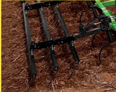
Heavy-duty coil tines on the 3-bar coil-tine harrow are 16 in. (406 mm) long and spaced 9 in. (229 mm) apart for smooth residue flow and excellent incorporation.
