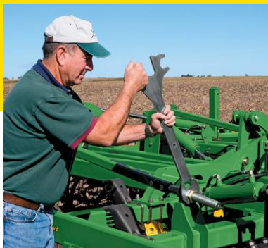
Side-to-side wing-leveling adjustments are easily made with a single adjustment bolt, located on top of the wing frame.
