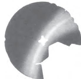
Disk fracture resulting from contact with rocks, stumps, or other solid objects. Credit is not offered.
