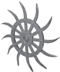
Sixteen curved tines on each wheel explode soil crust and uproot weeds. These wheels can also fit Yetter, M&W, and Hiniker rotary hoes.
