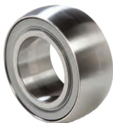
Maintenance free bearings are features of the new John Deere 2600 Series Disks. A high-density polymer liner allows the bearing to dynamically align the shaft in rough field conditions.
