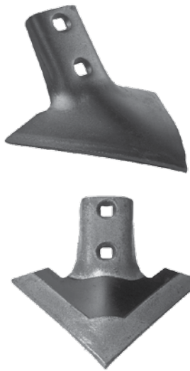
Examples of medium crown, 51-deg.-shank-angle conventional-wing sweeps for primary and seeding tillage.
