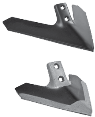
Examples of Tru-Width sweeps for primary and seeding tillage. Medium crown, 51-deg. shank angle.
