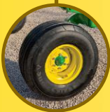
Radial Tires Standard equipment for mainframe wheels. Improves in-field and on-road transport, provides stubble resistance, reduces compaction and wears longer.
