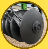
Disk Gang Provides aggressive cutting action to size up to 80% residue and minimizes ridging for a smooth and level seedbed profile.
