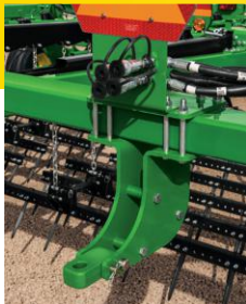
Rear hitch is compatible with all Level-lift and Floating Hitch configurations to provide more versatility with tow-behind attachments such as the John Deere 200 Seedbed Finisher. Tongue weight is improved to 1,500 lbs. (680 kg) 13,000 GVW rating.
