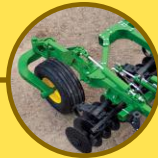
Active-Hydraulic Caster Wheels Help to maintain a consistent, level depth, recommended for operation on rolling ground or when the disk gangs are operated in the raised position.
