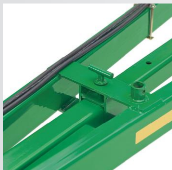
Tongue length adjustments can be made with a simple pin adjustment, making it easy to create the desired turning radius.
